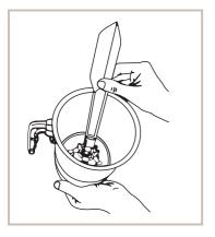
To fit the dry grinding blade on the shaft in the jar, hold the Nylon coupler on the underside of the jar with one hand, and with the help of the spanner (provided in the handle of the spatula) tighten by rotating it anti clockwise till the blade is securely fastened.
