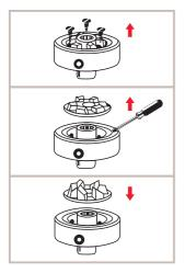
Unscrew the three screws located amidst the teeth of Driving Gear.
