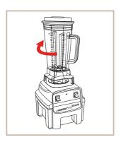
Place the Jar onto the Motor Unit firmly and turn clockwise to ensure that it locks properly.
