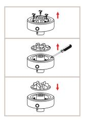
Unscrew the three screws located amidst the Teeth of Driving Gear
