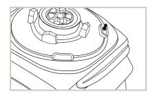
A Micro Switch has been provided on the top of the Motor Unit. It does not let the Motor start unless the Jar has been locked properly onto the locks provided on the Motor Unit and therefore provides safety against Jar falling of when the machine is ON.
