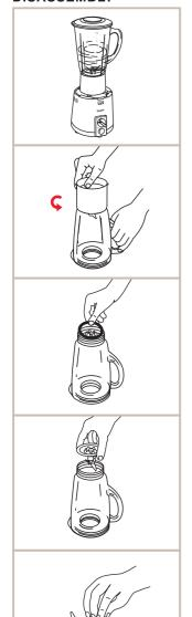
To clean the liquidiser jar quickly and thoroughly, fill the jar one third full of luke warm water and add a few drops of detergent or soap flakes. Switch the motor ON and run for some time. The soapy water will clean the jar. Switch off the motor and empty the blender jar.
