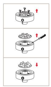
Unscrew the three screws located amidst the teeth of Driving Gear.
