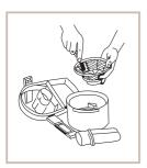
The plug should be disconnected. Follow instructions for disassembly of juicer. Rinse each part in cold or luke warm water. Cutter spinner also works as the filter, so rinse this especially well. After rinsing, wipe the water off and let it dry before storing.
