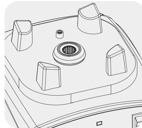
A Micro Switch has been provided on the top of the Motor Unit. It does not let the Motor start unless the Jar has been placed properly at the position provided on the Motor Unit and therefore providing safety against unwanted incidence.
