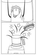
Plug into a convenient electrical outlet. Turn the speed control knob to 'HIGH' speed. Use 'HIGH' speed only for dry grinding and chutney grinding. Speed control knob can be rotated in clockwise direction only.
